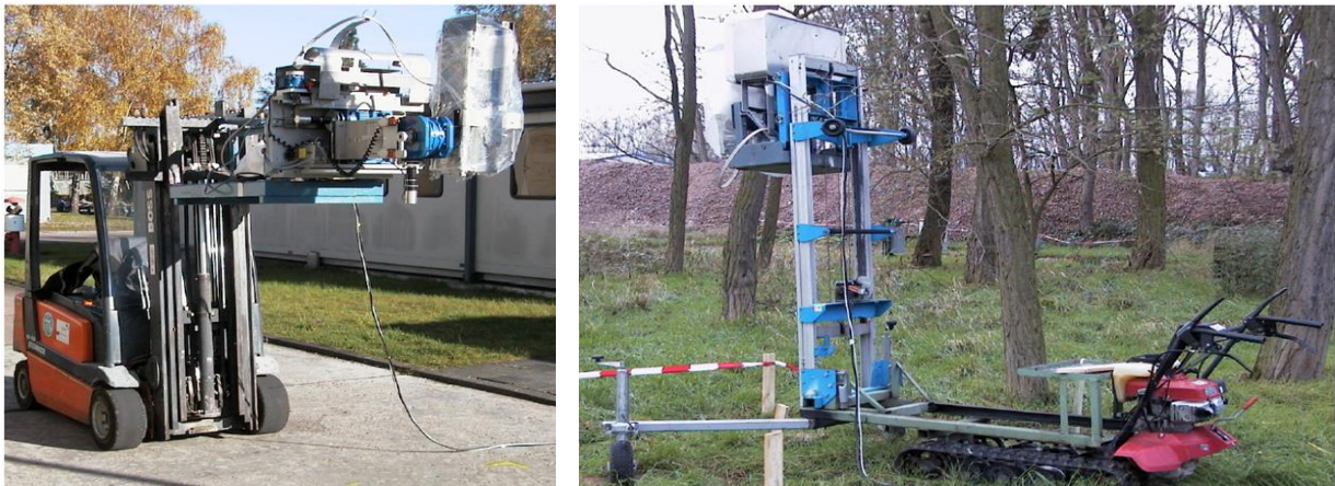
Figure 4-27: Gamma spectrometry of paved (left) and unsurfaced (right) external areas
