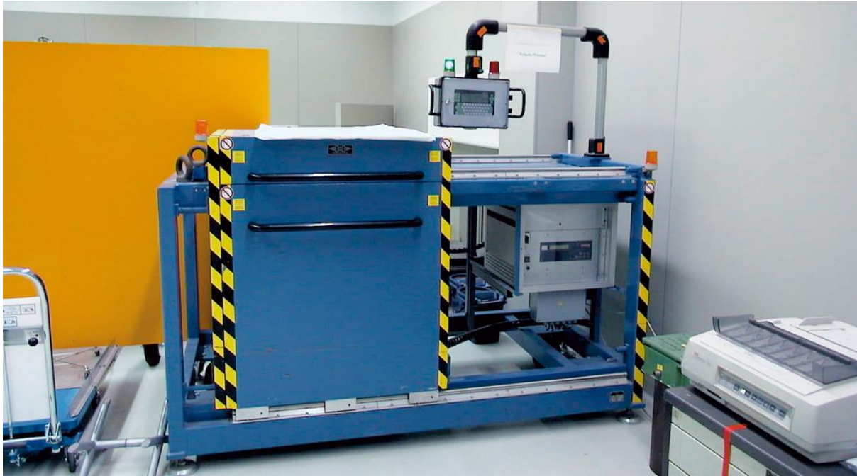
Figure 4-14: Free release measurement facility for components [reference Kahl NPP]
