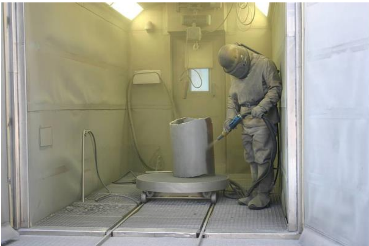
Figure 4-9: Dry blasting decontamination [reference EWN]
