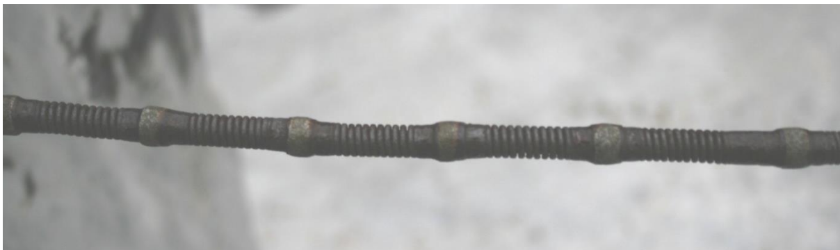
Figure 4-2: Cutting wire with diamond “pearls” and distance springs [reference Wikipedia]
