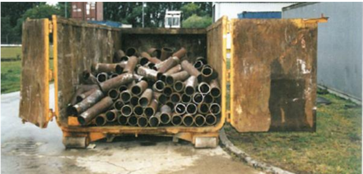
Figure 4-15: Free released metallic material for recycling [reference Kahl NPP]
